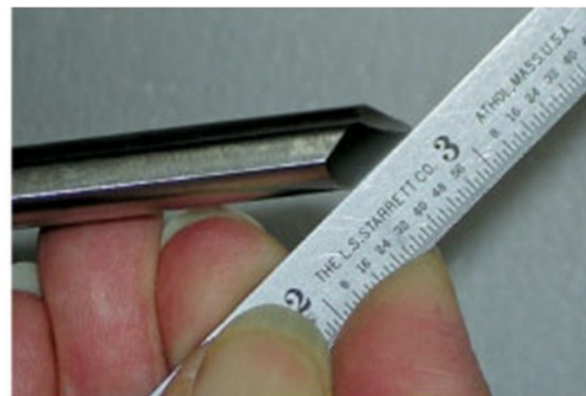
The bevel (grind) of a cutting tool should be flat
