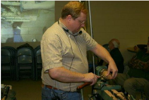
Cutting the outside shape with the right hand and gouge while holding the lid on with the left hand.
