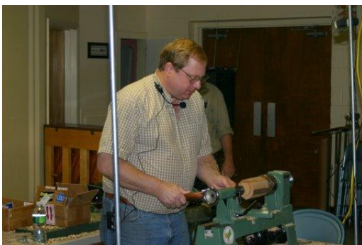
Cutting a tenon on the right.
