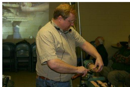
Turning the base with the lid attached to allow easy visualization of the outside shape.
