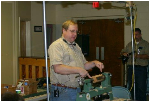
These ends get tenons for grabbing with the chuck.
