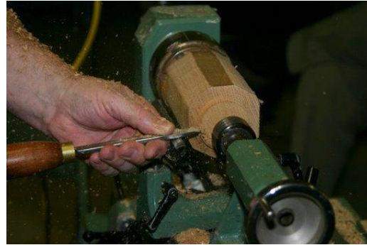
Cutting the tenon on the right—detail.
