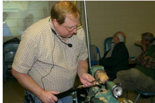
Lid reassembled to the vessel; turning the outside with tailstock support.
