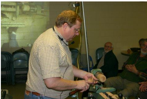
Refining the outside using two hands for control.
