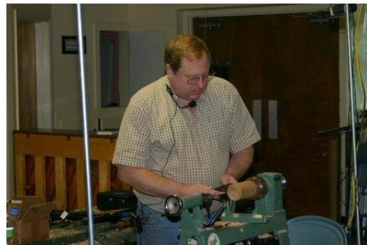
Slicing in two with a narrow parting tool.
